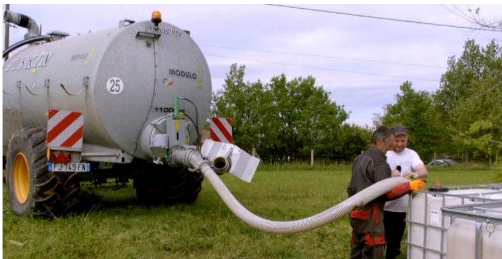
Figure 13 : pompage cuves IBC - 19/04/2024
